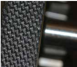
Proprietary synchronizer friction material (EFM-H) improves abuse resistance by more than 200%.
